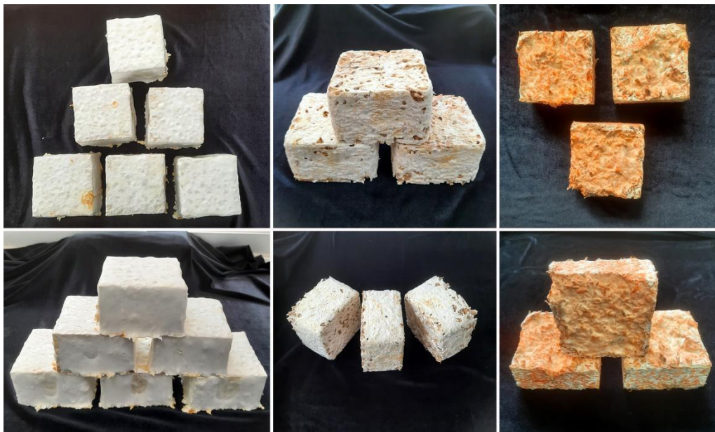
Fig. 5 – Mushroom mycelium pre-composite blocks prepared with different combinations of mushroom strains and substrates.
